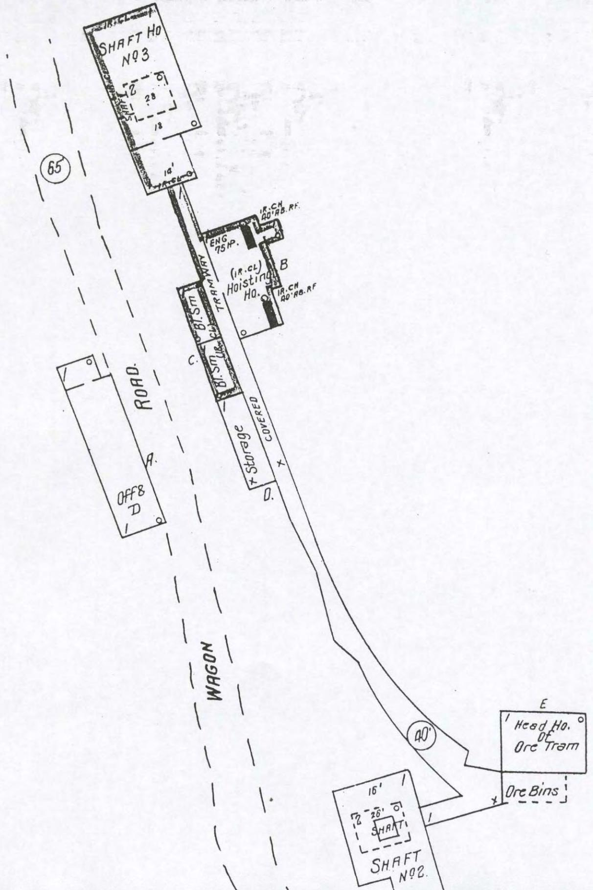
When the Amethyst company expanded the surface plant in the late 1890s, mine workers removed or buried many of the facilities associated with the original shaft house. The original hoist foundation, the blacksmith and carpentry shop areas, the rail line, and shaft house foundations are missing from extant remains.
