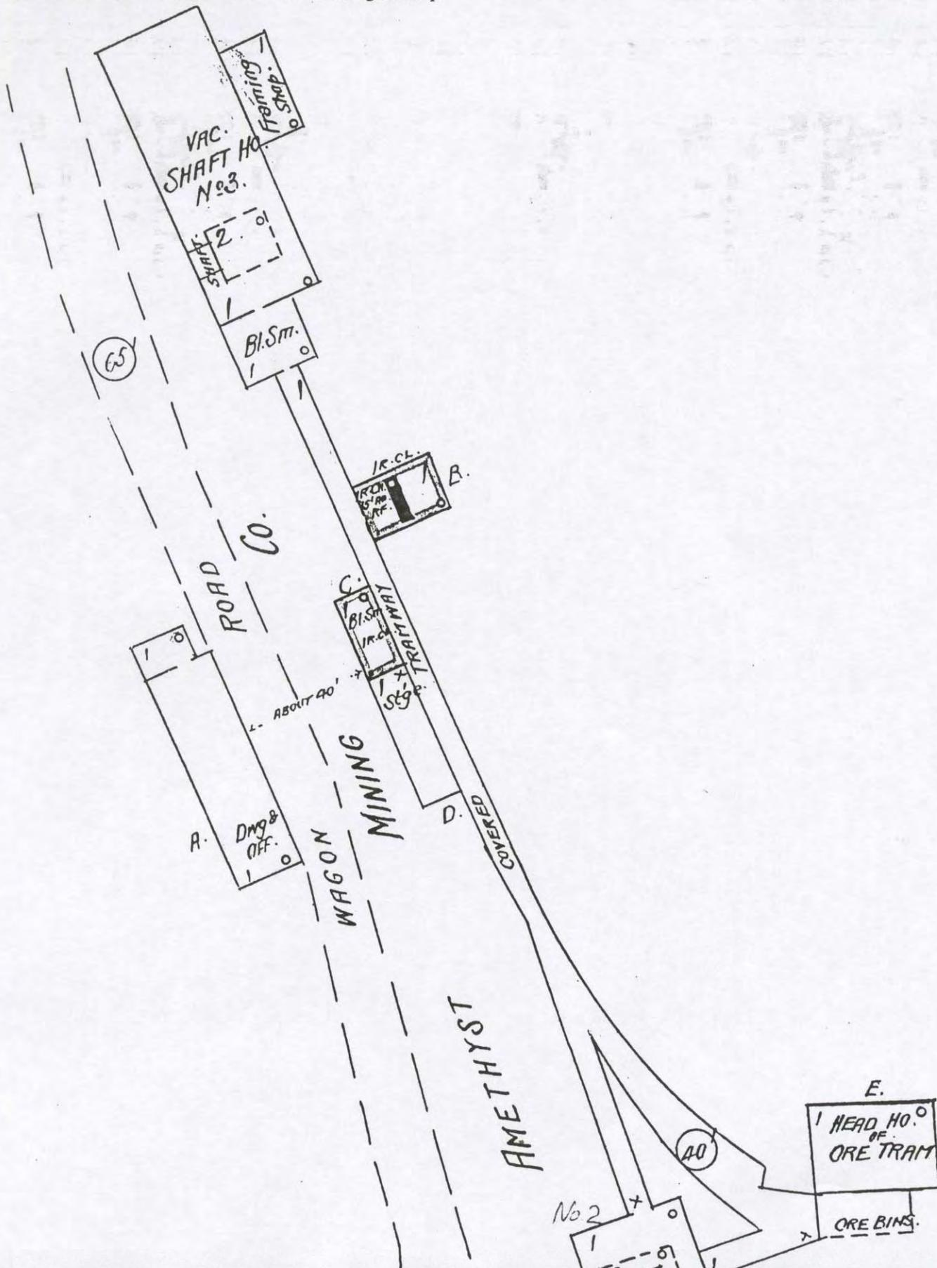
Figure 7.8 Sanborn's 1904 map of the surface plants associated with shafts No.2 and No.3. The hoist house and shops for Shaft No.3 have been enlarge. To scale with the archaeological map.
