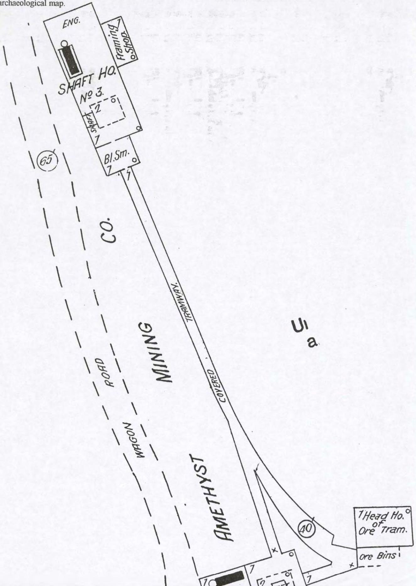
Figure 7.7 Sanborn's 1898 map of the surface plants associated with shafts No.2 and No.3. Note that the machinery for Shaft No.2 has been removed, and that a hoist house and shops have been added to the plant for Shaft No.3. To scale with the archaeological map.
