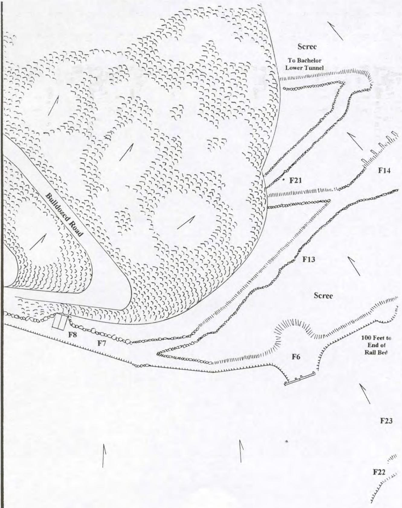
The site's material remains indicate that the late 1890s surface plant included an explosives magazine and a timber dressing shop. The magazine (Feature 8) still stands, and it is a well-built front-gabled structure. Mine workers erected the building, which 8 by 8 feet in area and 10 feet high, on a platform consisting of sorted gravel fill retained by a dry-laid rock wall. The structure is composed of corrugated iron siding nailed to a 2x4 post-and-girt frame.
